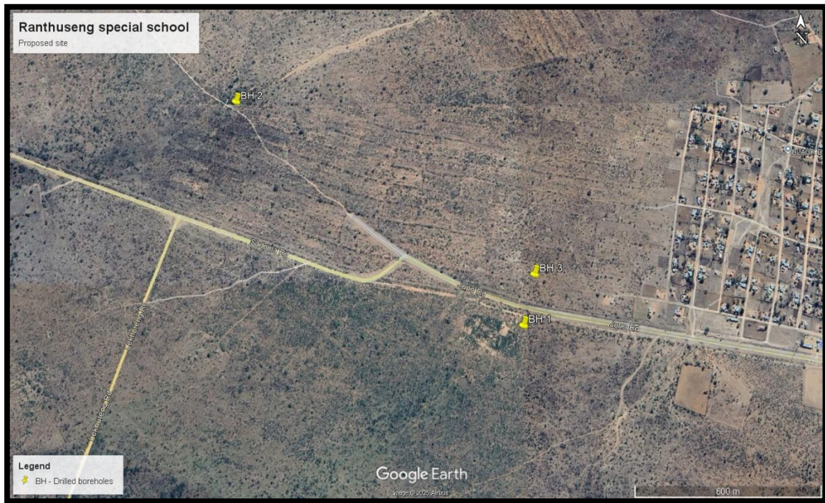
Figure 10: New drilled boreholes within the proposed site
